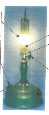
Alcohol cup. This was filled with alcohol and lit to warm up the mantles when preparing to light the lamp.
